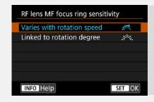
When paired with the EOS R or EOS RP, users can select from two manual focus ring sensitivity options: "Varies with rotation speed" and "Linked to rotation degree". (Left: EOS R camera menu)
